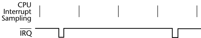
Figure 9-7: Short interrupt request pulses require edge sensitive input.
